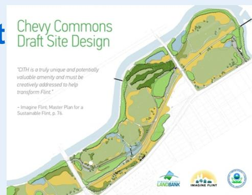
The plan calls for the site to be capped with an attractive low-maintenance natural landscape intended to minimize maintenance and storm water management costs. Details on the first three proposed phases are included in the design plan.
